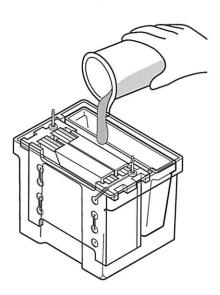
7. Add a standard stir bar to help maintain even buffer temperature and ion distribution in the tank. Set the speed as fast as possible to keep ion distribution even.
