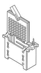
6. Add the frozen Bio-Ice cooling unit. Place in tank and completely fill the tank with buffer.
